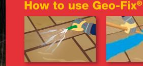
Step 1 Wet entire area to be jointed. Use a hosepipe with a hose nozzle or a watering can with rose.
